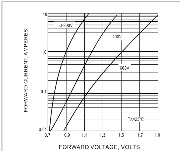
Fig.3 FORWARD CHARACTERISTICS
