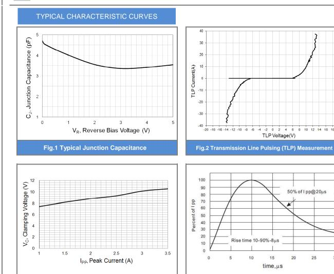
Fig.3 Typical Peak Clamping Voltage(8/20µs)
